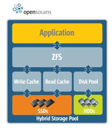
Figure 3. ZFS transparently optimizes data placement across hard disk drives and SSDs to deliver improved throughput.
