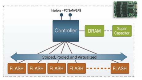
Figure 2. Enterprise solid state drive high-level architecture
