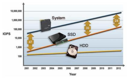
Figure 4. CPU, Flash, and hard disk drive technology advancement trends
