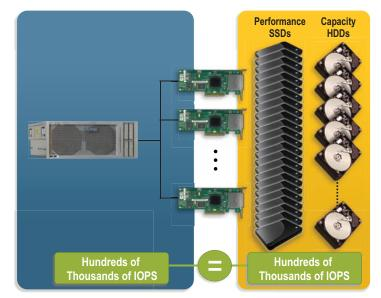
Figure 5. The hybrid storage pool provides a tiered architecture that lets data be placed on the right kind of device to balance system performance
