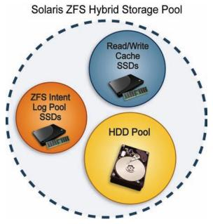
Figure 6. Solaris ZFS automates storage management and helps balance system performance with the ZFS Intent Log, a read cache, and a high capacity storage pool
